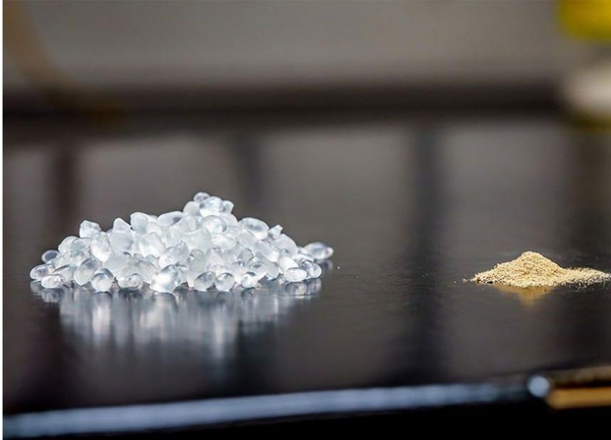
The biodegradable "living plastic" is made by combining thermoplastic polyurethane (TPU) pellets (left) and *Bacillus subtilis* spores (right) that have been engineered to survive the high temperatures used to produce the plastic.
