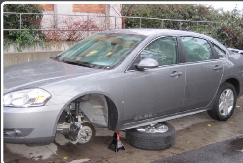
To test the electronic control unit (ECU) in a controlled environment, the researchers immobilized the car on jack stands while mounting attacks.
